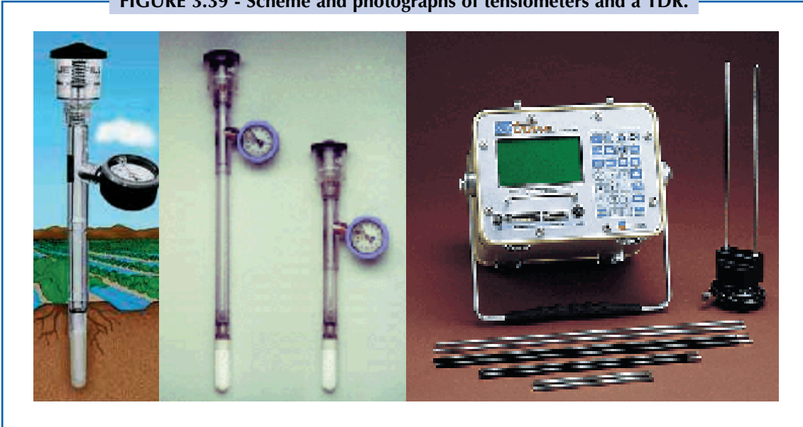
FIGURE 3.39 - Scheme and photographs of tensiometers and a TDR.
