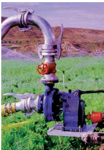
FIGURE 3.46 - Left: a rotodynamic pump powered by a tractor. Right: a pumping unit with rotodynamic pumps in parallel.
