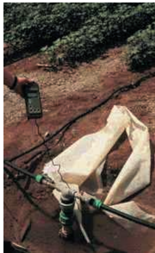
FIGURE 3.40 - Measurement of irrigation water with a conductivity meter.
