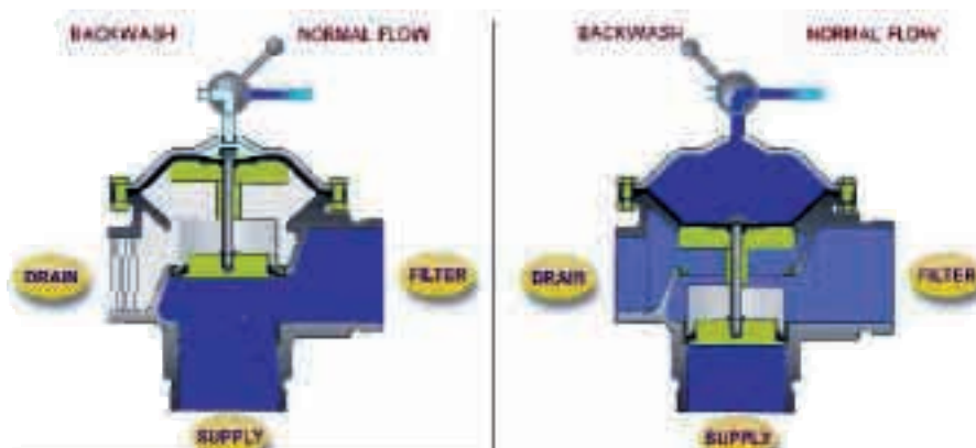
FIGURE 3.21 - An automatic self-cleaning filter uses the back flushing mechanism for the removal of accumulated debris.
