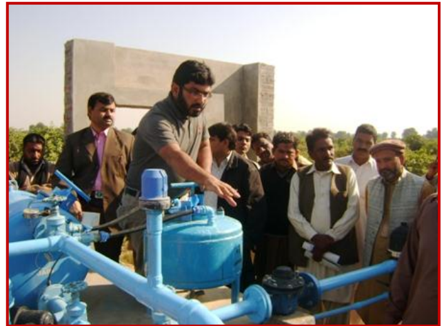
Representative of SSC explaining the farmers about maintenance of the drip system
