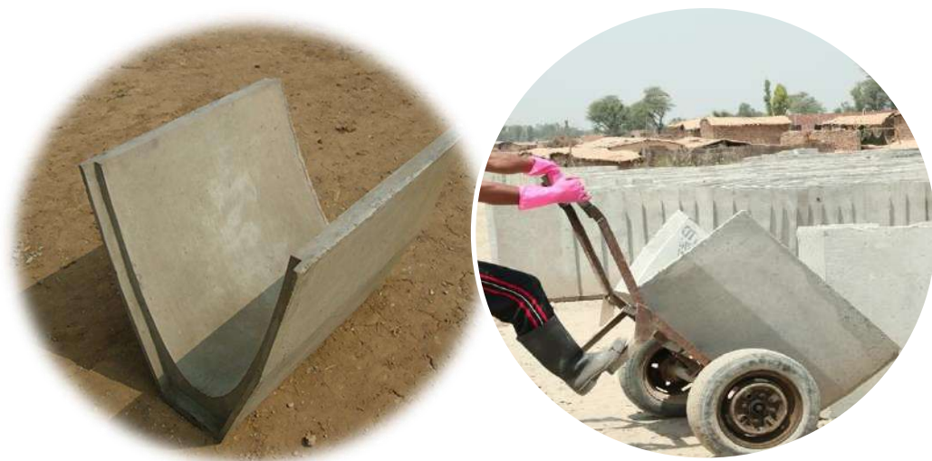
Figure 1. Precast Concrete Parabolic Segments (PCPS)
